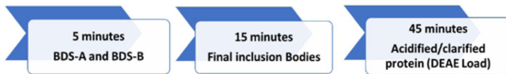
Figure 6: Cleaning time of process soils with 2% v/v alkaline detergent at 80°C.
