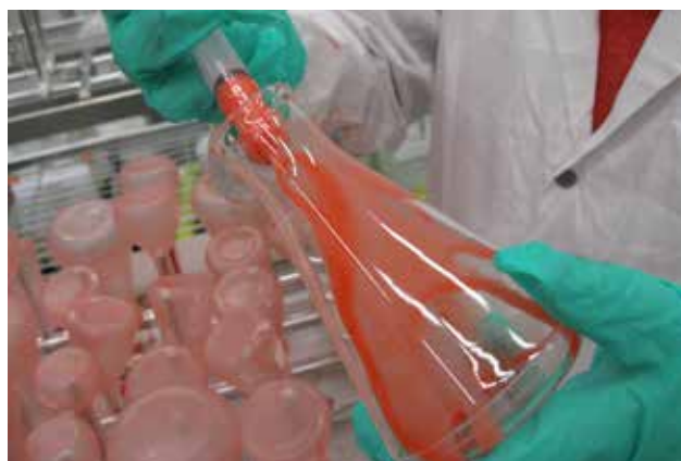
Figure 1: Master soil (Browne soil) applied to laboratory glassware. Browne residue is similar to the Edinburgh soil used to simulate the residue observed naturally during hospital surgical procedures.
