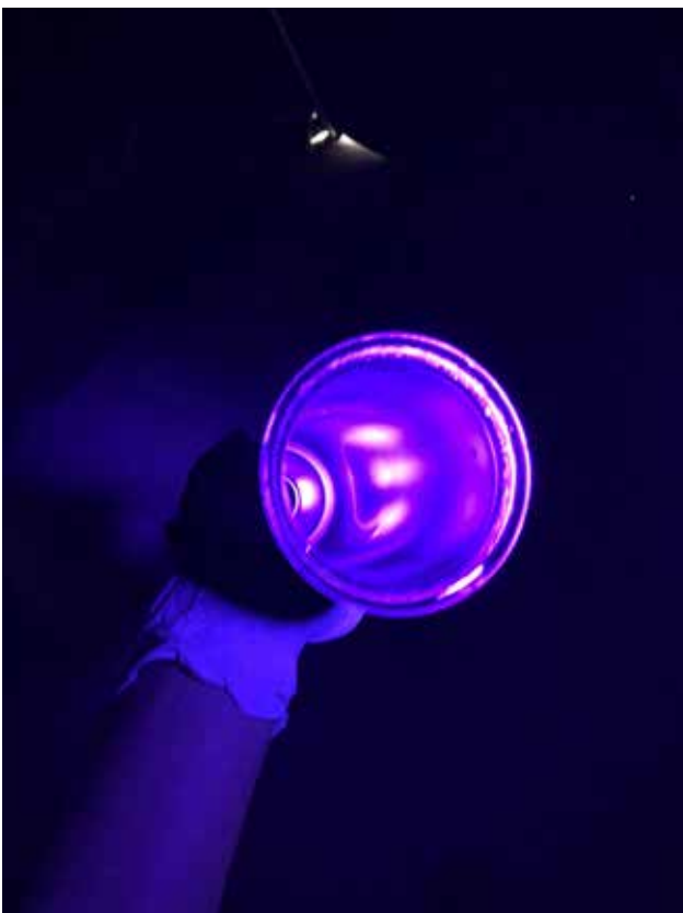
Figure 5: Inspection of filter housing under UV light for traces of riboflavin.
